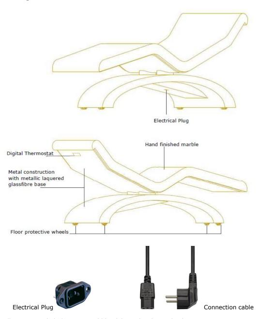
If fixed installation is needed Cleopatra could be delivered without wheels. In this case the connection could be be hidden in the base.
